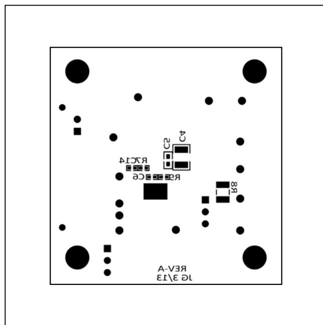
Figure 7. MAX16936 EV Kit Component Placement Guide—
