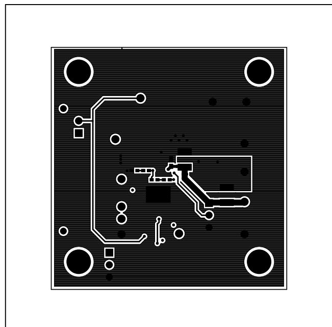
Figure 6. MAX16936 EV Kit PCB Layout—Solder Side
