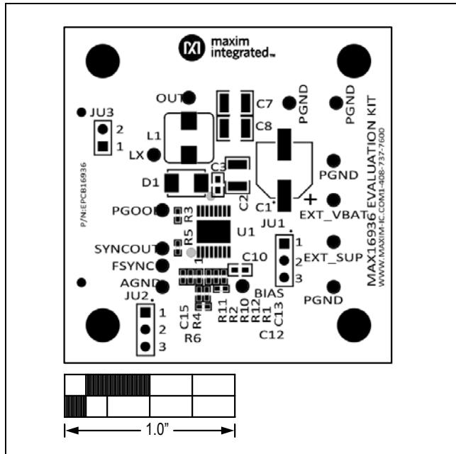
Figure 2. MAX16936 EV Kit Component Placement Guide—Component Side
