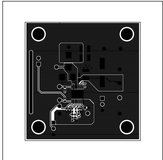
Figure 3. MAX16936 EV Kit PCB Layout—Component Side
