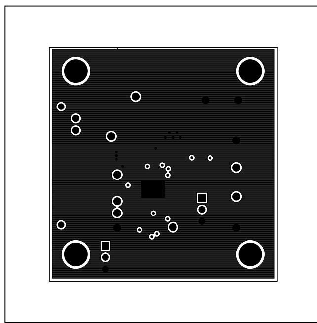
Figure 4. MAX16936 EV Kit PCB Layout—Layer 2
