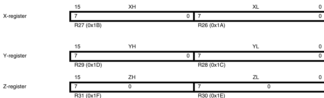
Figure 12-3. The X-, Y-, and Z-registers
