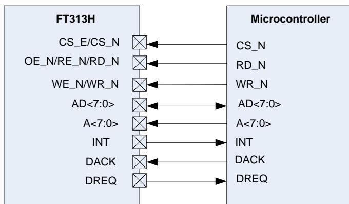
8-Bit SRAM bus interface doesn't use high AD<15:8> data bus, must terminate AD<15:8> signals with external 10k ohm pull-down resistors.
