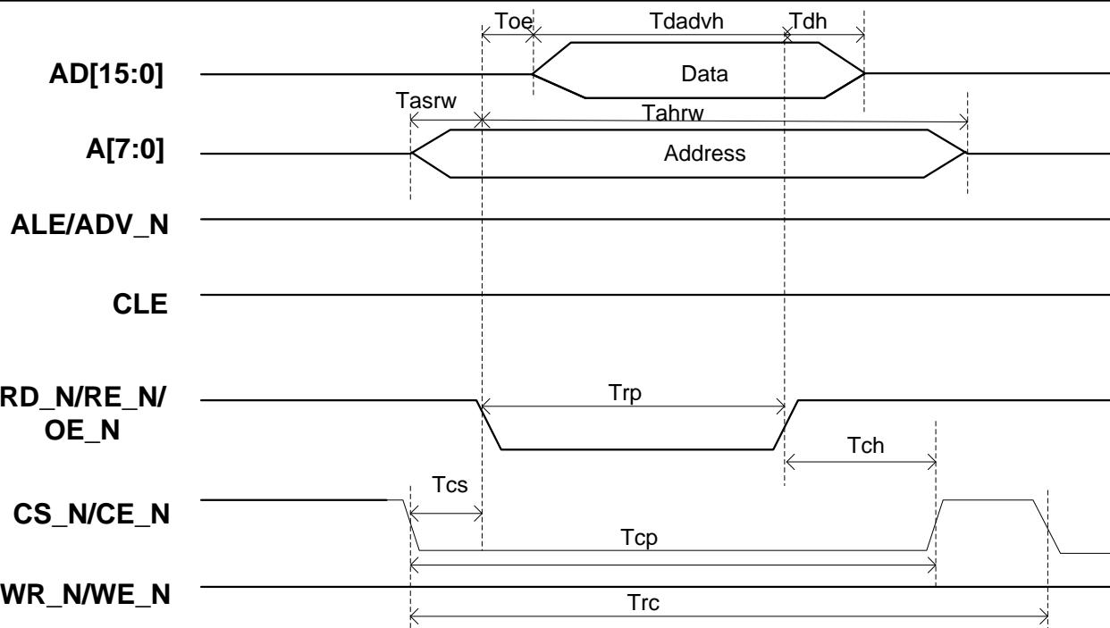
**Figure 6-1 Read in SRAM mode**
