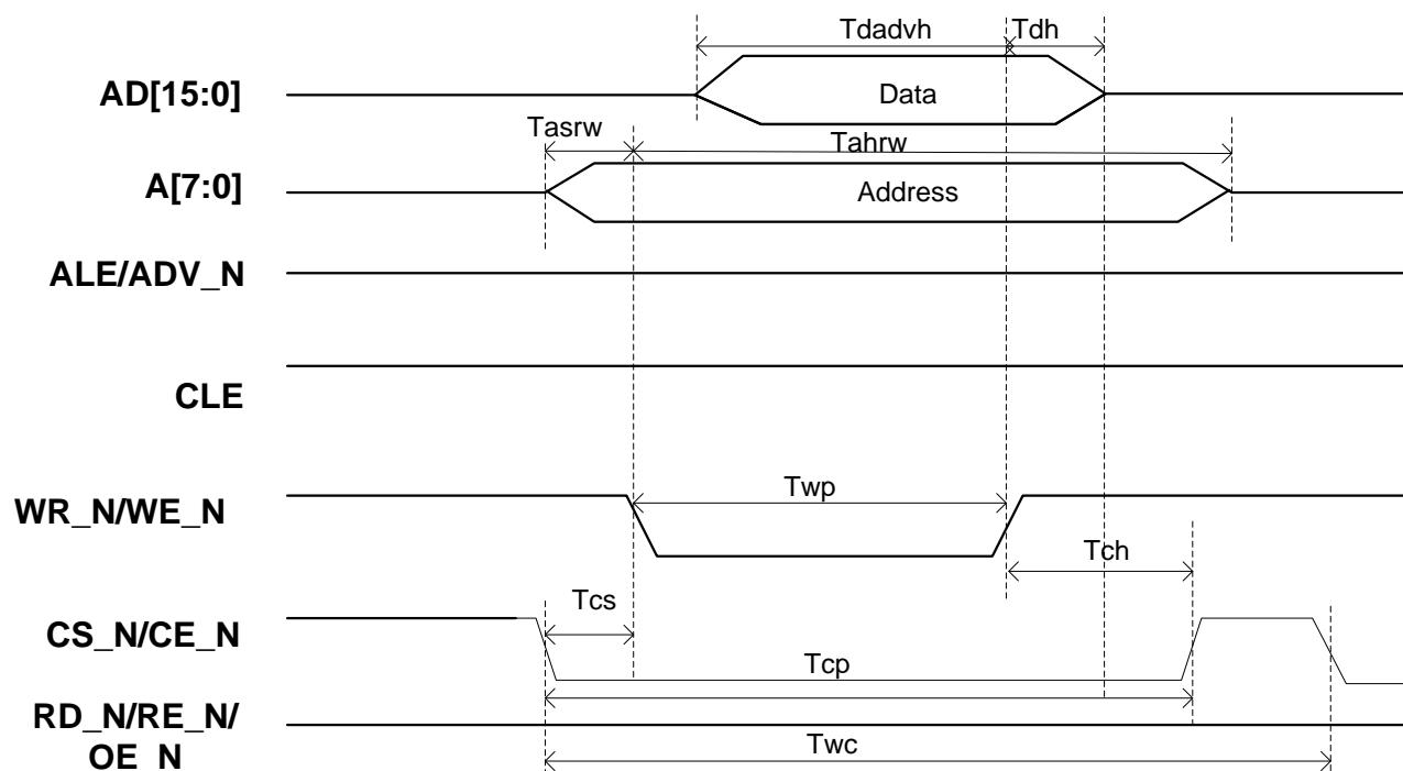
**Figure 6-2 Write in SRAM mode**
