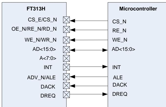
16-Bit General Multiplex uses AD<15:0> signals as address and data bus. Unused A<7:0> address must be terminated with external 10k ohm pull-down resistor.
