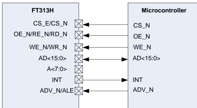
16-Bit NOR uses AD<15:0> signals as address and data bus. Unused A<7:0> address must be terminated with external 10k ohm pull-down resistor.
