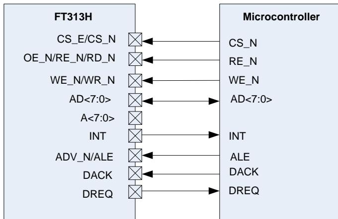
8-Bit General Multiplex uses AD<7:0> signals as address and data bus. The unused high data bus AD<15:8> and A<7:0> address bus must be terminated with external 10k ohm pull-down resistors.
