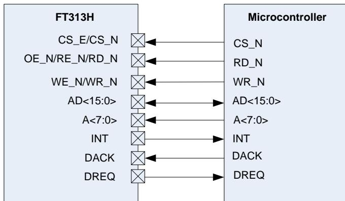
If DMA transfers are not used the DACK and DREQ signals may be left floating or the DACK signal may be terminated with external 10k ohm pull-down resistor.
