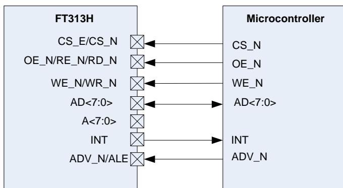
8-Bit NOR uses AD<7:0> signals as address and data bus. The unused high data bus AD<15:8> and A<7:0> address bus must be terminated with external 10k ohm pull-down resistors.
