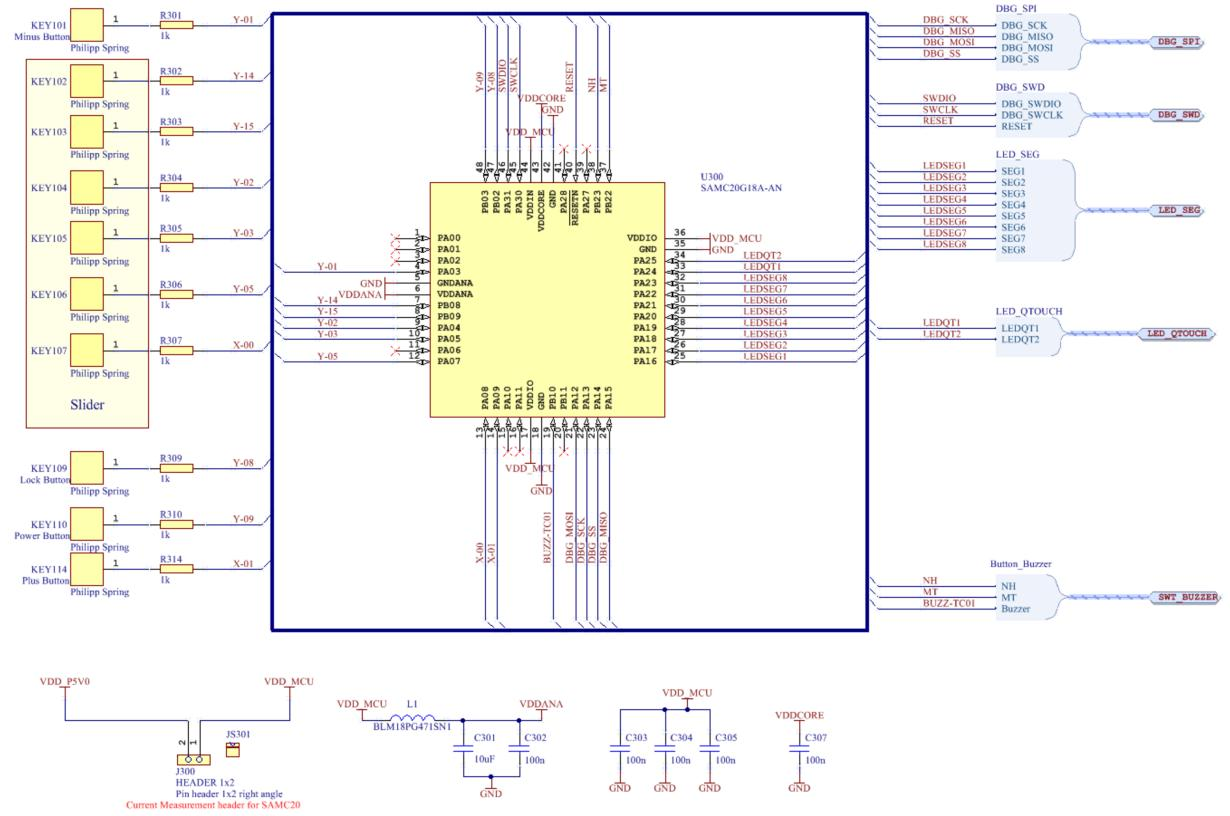
**Figure 11-2 LED Segment, Buzzer, and Switch Section**
