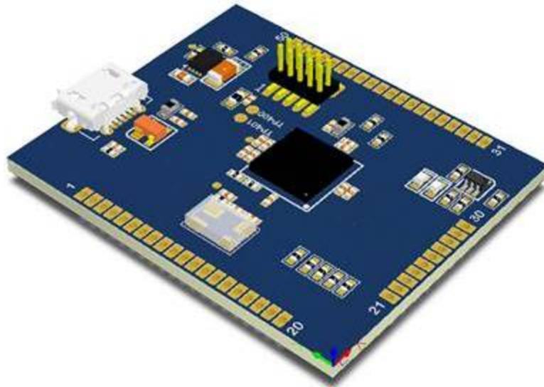
The EDBG is mounted on the kit as a separate module. Using the EDBG the user can connect to a QTouch Analyzer and view the touch data. The EDBG has been pre-configured to support a SAMC20G18 device using SWD interface for programming and debugging. For streaming data to the QTouch Analyzer it uses DGI, which connects to SAM C20 over Bit Bang SPI.
