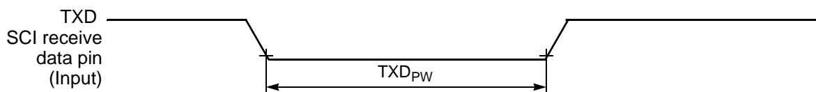
Figure 10-13 TXD Pulse Width
