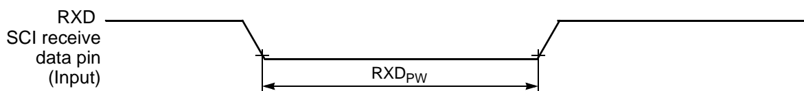
Figure 10-12 RXD Pulse Width
