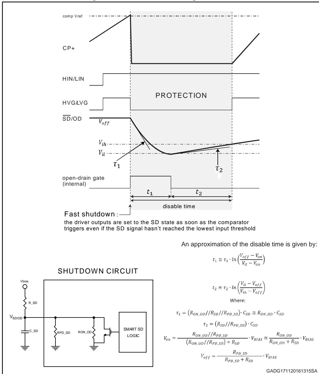
Please refer to [Table 13: "Sense comparator characteristics \( \$V\_{CC} = 15\$  V unless otherwise specified\)"](#) for internal propagation delay time details.
