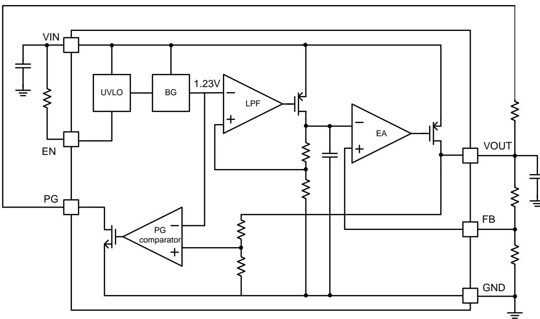
Figure 1—Block Diagram of Super Low Dropout Regulation
