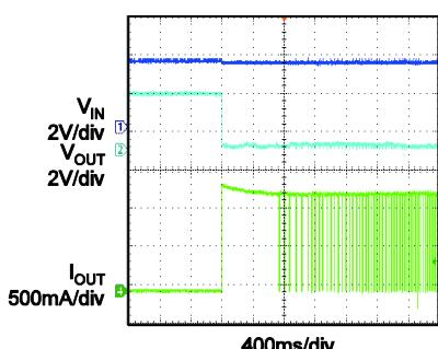
**TYPICAL PERFORMANCE CHARACTERISTICS (continued)** $V_{IN}=3.3V$ ,  $V_{OUT}=2.8V$ ,  $C_{IN}=C_{OUT}=2.2\mu F$ ,  $T_A=25^\circ C$ , unless otherwise noted**Over Current Protection
