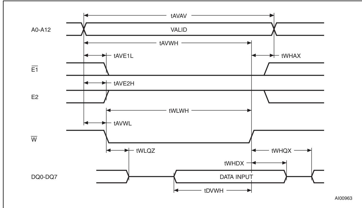
**Figure 7.** Chip enable controlled, WRITE AC waveforms
