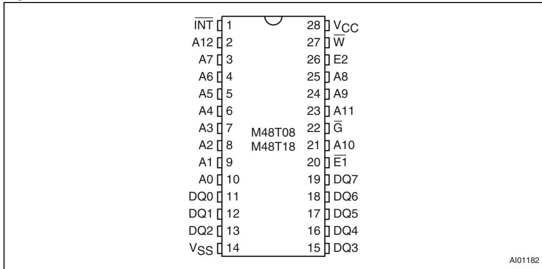
**Figure 3. SOIC connections**
