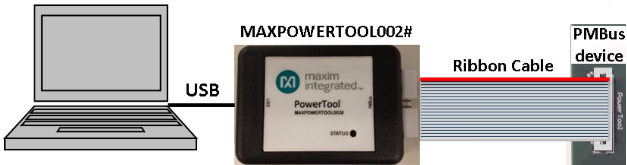
Figure 1. MAXPOWERTOOL002# Installation
