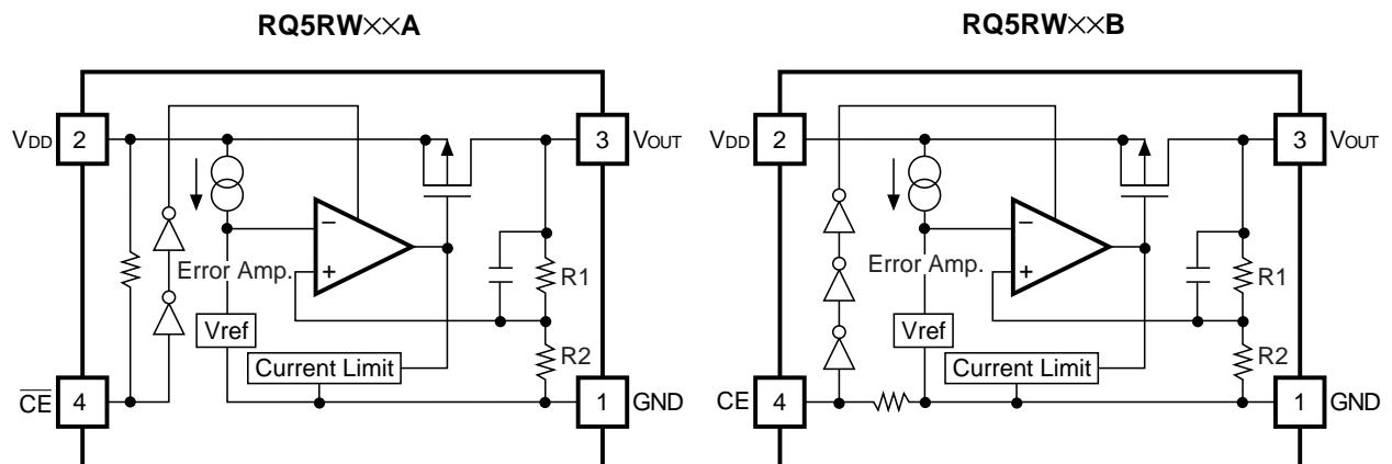
In these ICs, Output Voltage  $V_{OUT}$  is detected by Feed-back Registers  $R_1$ ,  $R_2$ , and the detected Output Voltage is compare with a reference voltage by Error Amplifier, so that a constant voltage is output.
