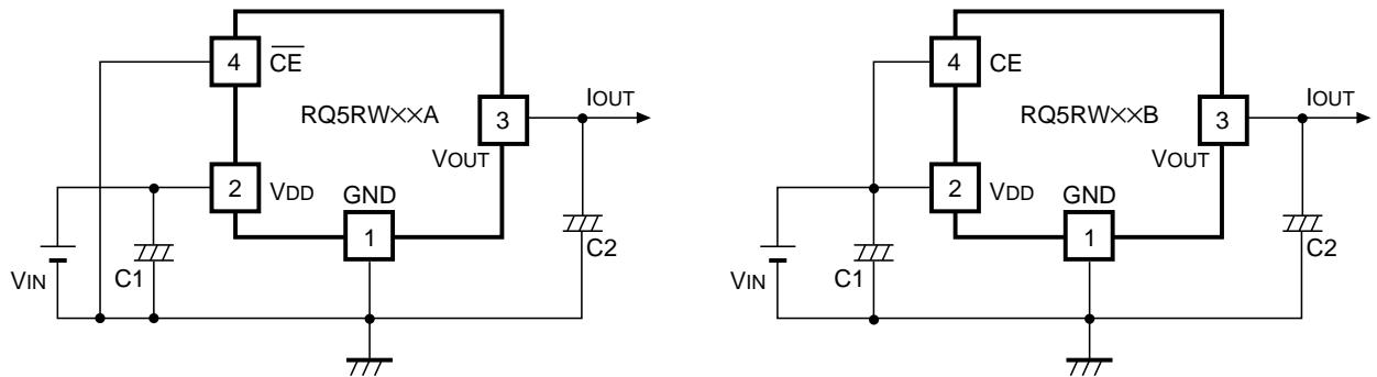
In RQ5RW Series, a constant voltage can be obtained without using Capacitor C1 and C2. However, when the wire connected VIN is long, use Capacitor C1. Output noise can be reduced by using Capacitor 2.
