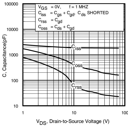
**Fig 5.** Typical Capacitance vs.
