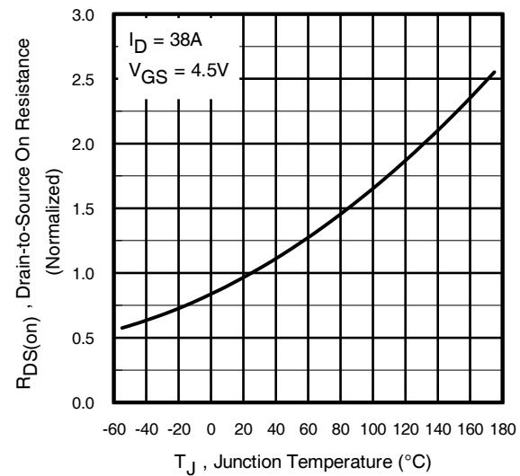
**Fig 10.** Normalized On-Resistance
