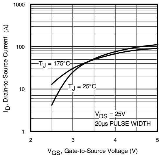
**Fig. 3** Typical Transfer Characteristics
