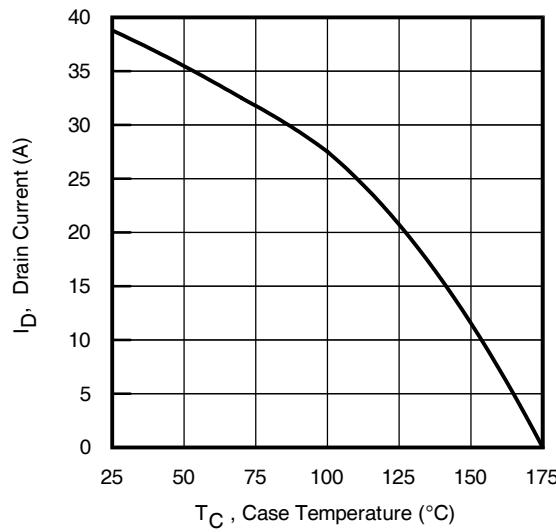
**Fig 9.** Maximum Drain Current Vs.
