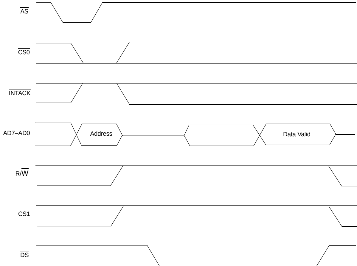
Figure 24. Read Cycle Timing
