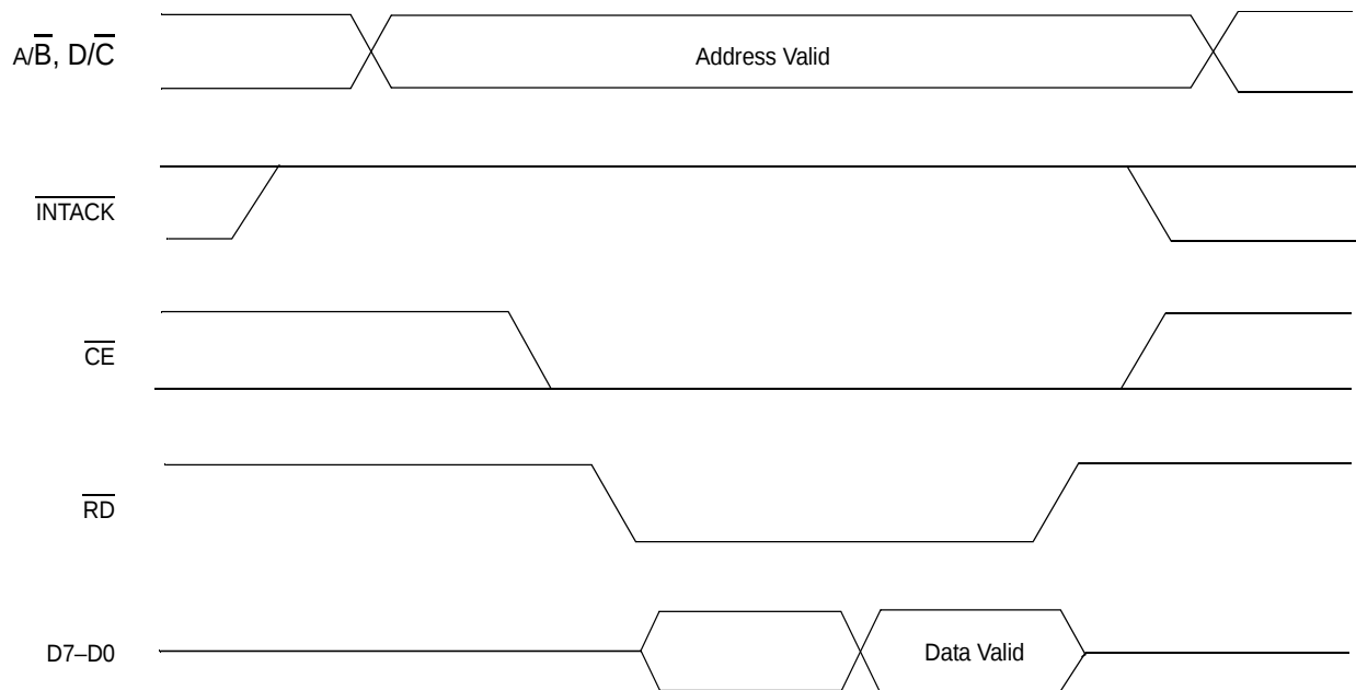
Figure 21. Read Cycle Timing
