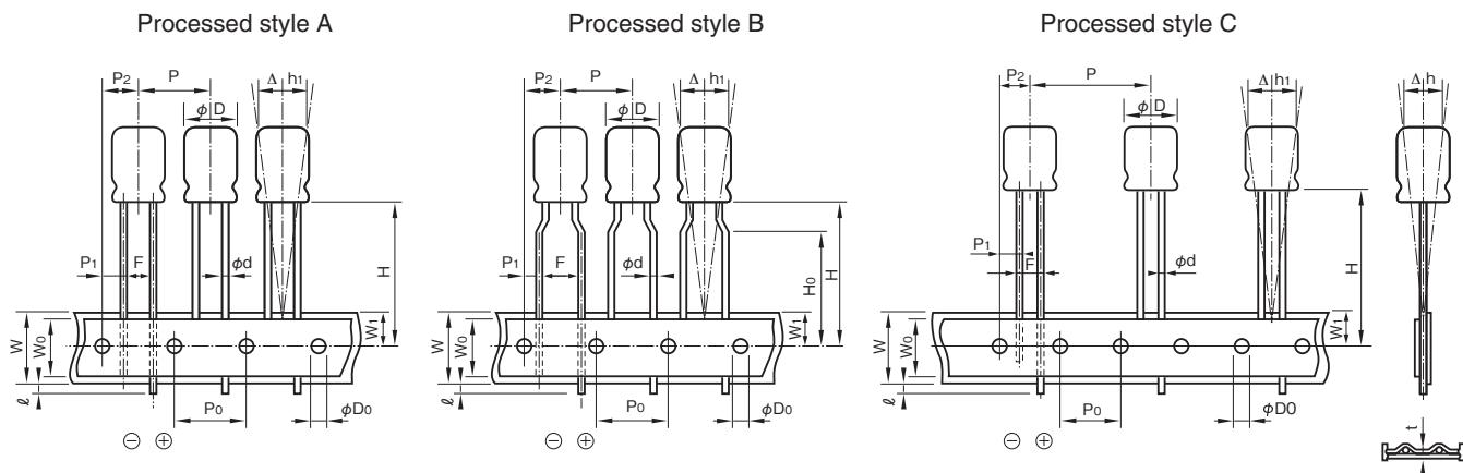
\*The shape of a lead wire sandwiched by the mounting strips may differ from the ones shown in the figures.
