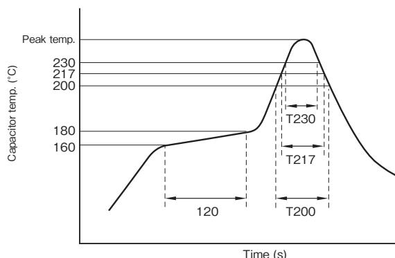
1. Preheating shall be under  $180^{\circ}\text{C}$  within 120 seconds.
