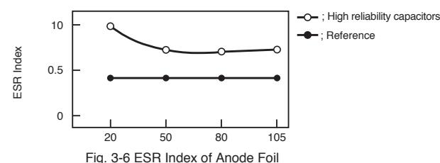
Fig. 3-6 ESR Index of Anode Foil
