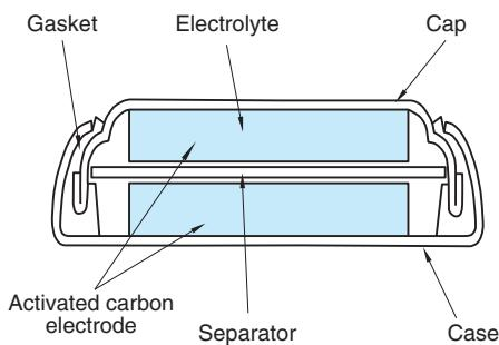
Fig.2 Example of Basic Construction of Coin Cell
