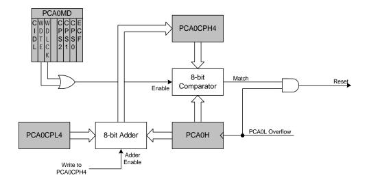
Figure 18.10. PCA Module 4 with Watchdog Timer Enabled
