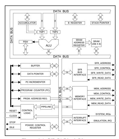
Figure 8.1. CIP-51 Block Diagram
