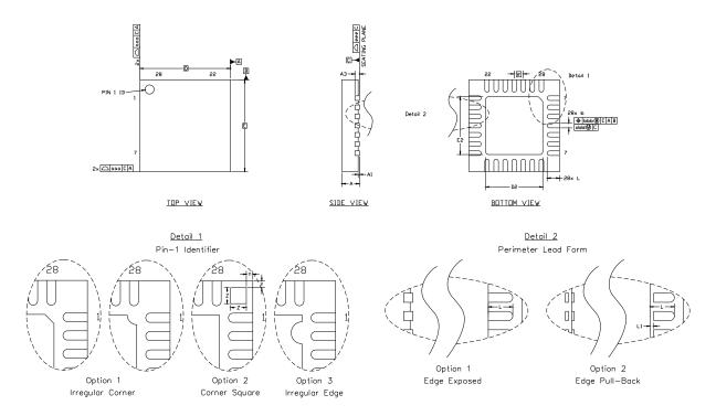
Figure 4.5. QFN-28 Package Drawing
