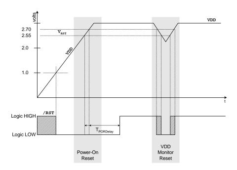
Figure 9.2. Power-On and V<sub>DD</sub> Monitor Reset Timing
