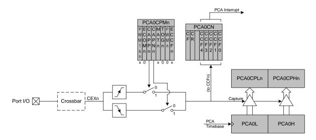
Figure 18.4. PCA Capture Mode Diagram
