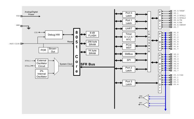
Figure 1.5. C8051F314 Block Diagram
