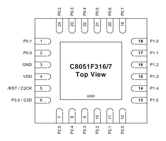
Figure 4.7. QFN-24 Pinout Diagram (Top View)
