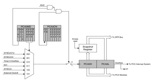
Figure 18.2. PCA Counter/Timer Block Diagram
