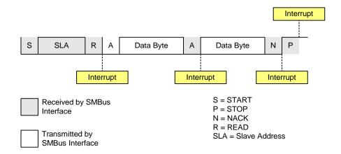
Figure 14.8. Typical Slave Transmitter Sequence
