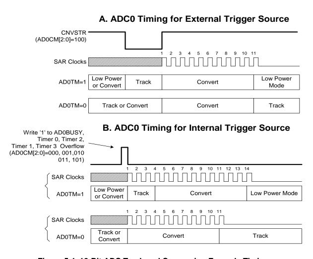
Figure 5.4. 12-Bit ADC Track and Conversion Example Timing
