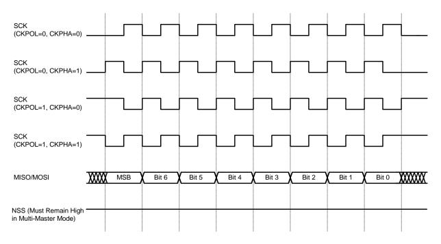
Figure 16.5. Master Mode Data/Clock Timing
