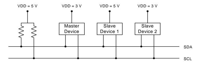
Figure 14.2. Typical SMBus Configuration
