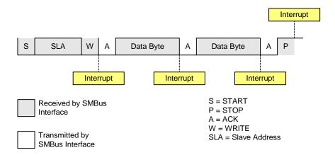
Figure 14.7. Typical Slave Receiver Sequence
