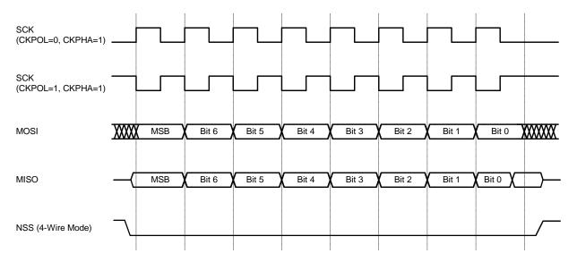
Figure 16.7. Slave Mode Data/Clock Timing (CKPHA = 1)
