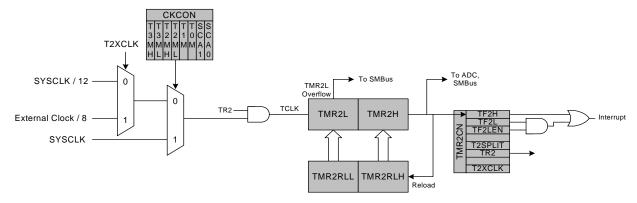
Figure 17.4. Timer 2 16-Bit Mode Block Diagram
