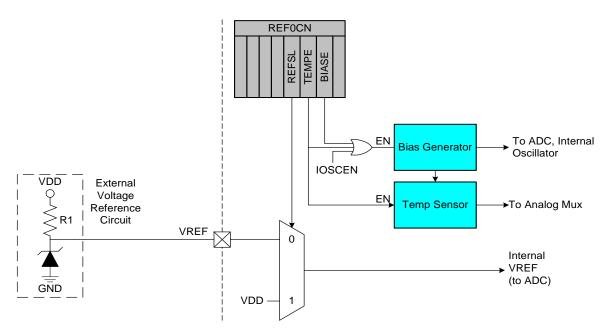
Figure 6.1. Voltage Reference Functional Block Diagram
