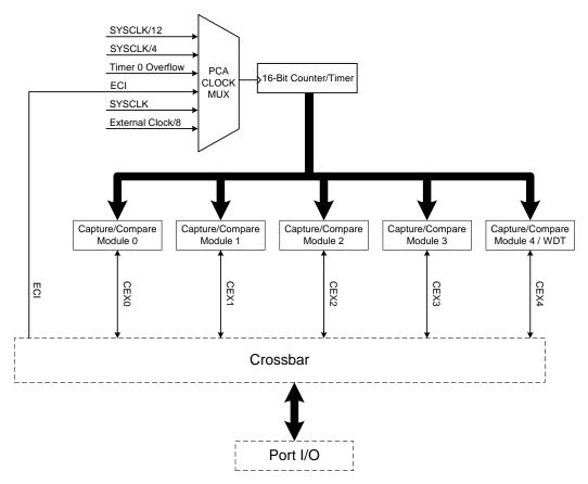
Figure 1.14. PCA Block Diagram
