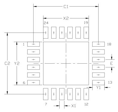
Figure 4.9. Typical QFN-24 Landing Diagram
