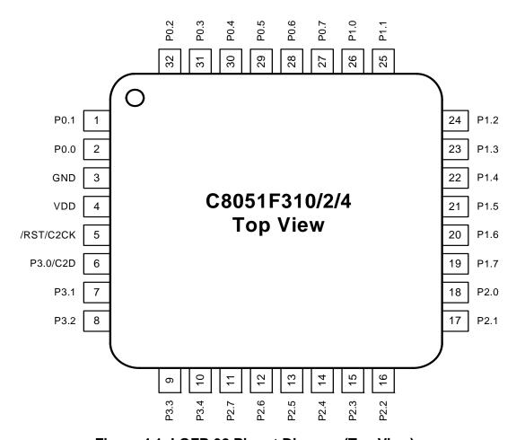
Figure 4.1. LQFP-32 Pinout Diagram (Top View)
