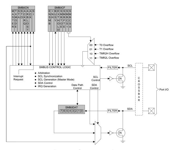
Figure 14.1. SMBus Block Diagram
