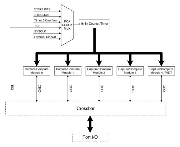
Figure 18.1. PCA Block Diagram
