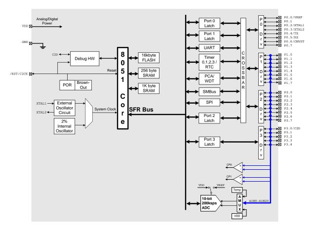
Figure 1.1. C8051F310 Block Diagram
