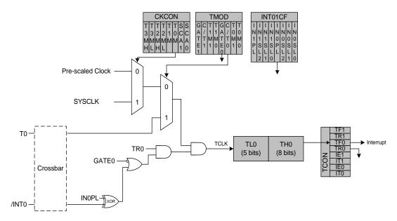
Figure 17.1. T0 Mode 0 Block Diagram
