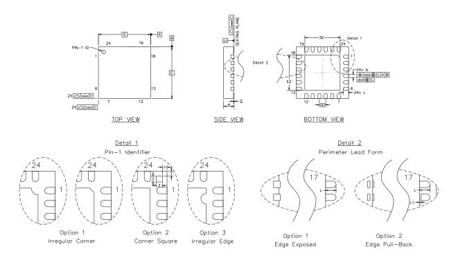
Figure 4.8. QFN-24 Package Drawing
