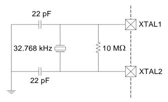
Figure 12.2. 32.768 kHz External Crystal Example
