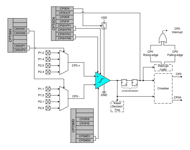
Figure 1.16. Comparator Block Diagram
