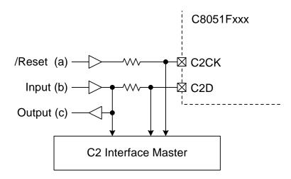
Figure 20.1. Typical C2 Pin Sharing
