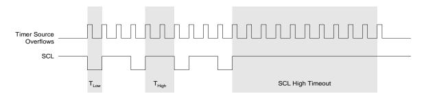
Figure 14.4. Typical SMBus SCL Generation
