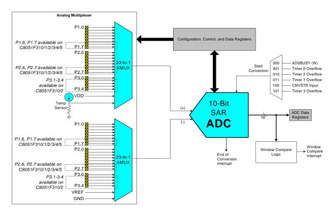
Figure 1.15. 12-Bit ADC Block Diagram
