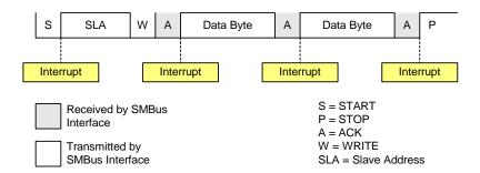
Figure 14.5. Typical Master Transmitter Sequence
