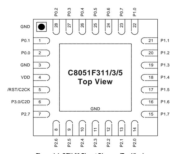
Figure 4.4. QFN-28 Pinout Diagram (Top View)
