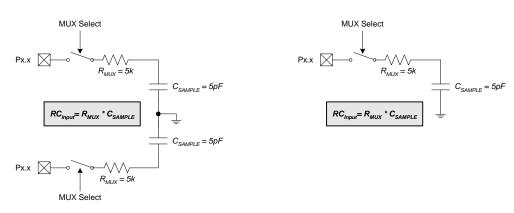
Figure 5.5. ADC0 Equivalent Input Circuits
