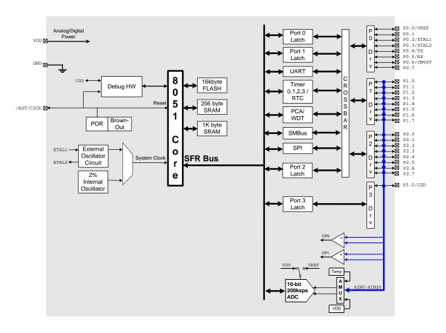
Figure 1.2. C8051F311 Block Diagram
