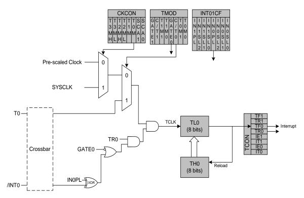
Figure 17.2. T0 Mode 2 Block Diagram
