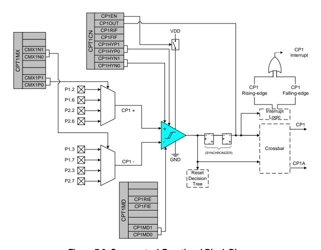
Figure 7.2. Comparator1 Functional Block Diagram
