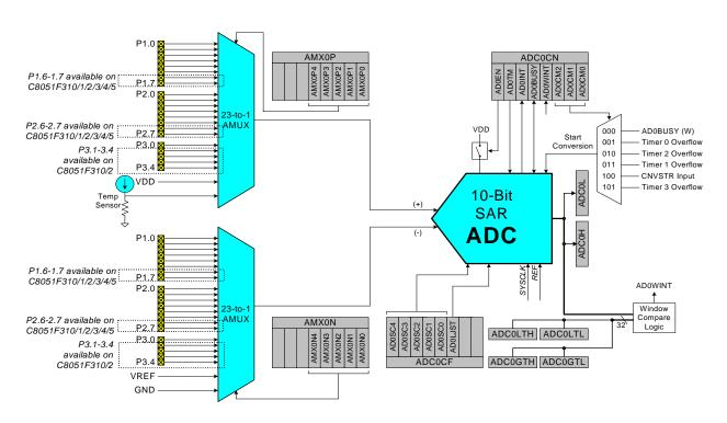
Figure 5.1. ADC0 Functional Block Diagram
