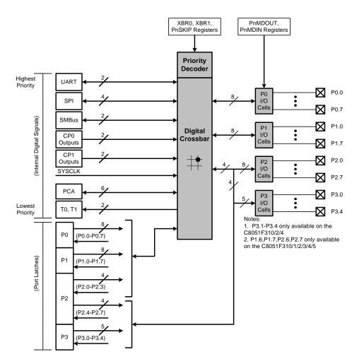
Figure 13.1. Port I/O Functional Block Diagram
