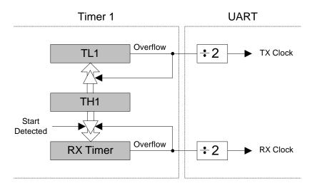
Figure 15.2. UARTO Baud Rate Logic
