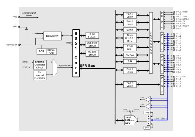
Figure 1.3. C8051F312 Block Diagram
