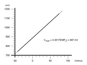
Figure 5.2. Typical Temperature Sensor Transfer Function
