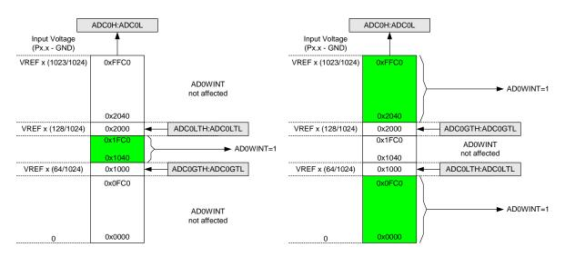
Figure 5.7. ADC Window Compare Example: Left-Justified Single-Ended Data
