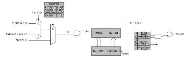
Figure 17.6. Timer 3 16-Bit Mode Block Diagram
