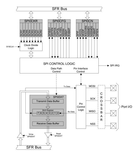
Figure 16.1. SPI Block Diagram
