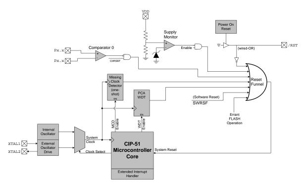
Figure 1.10. On-Chip Clock and Reset
