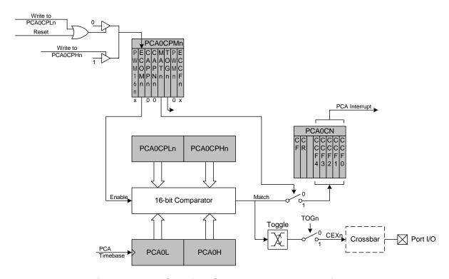
Figure 18.6. PCA High Speed Output Mode Diagram
