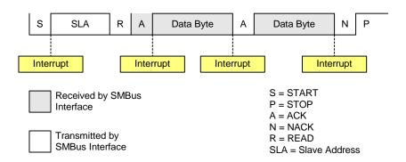
Figure 14.6. Typical Master Receiver Sequence
