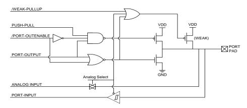
Figure 13.2. Port I/O Cell Block Diagram
