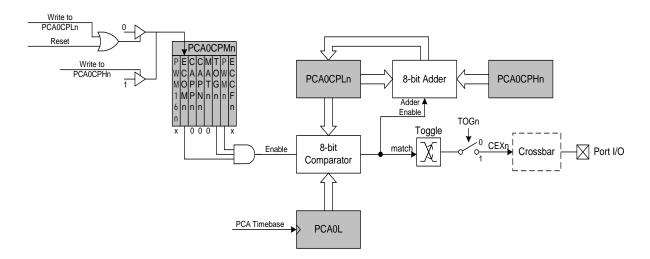
Figure 18.7. PCA Frequency Output Mode
