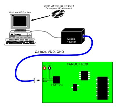
Figure 1.12. Development/In-System Debug Diagram
