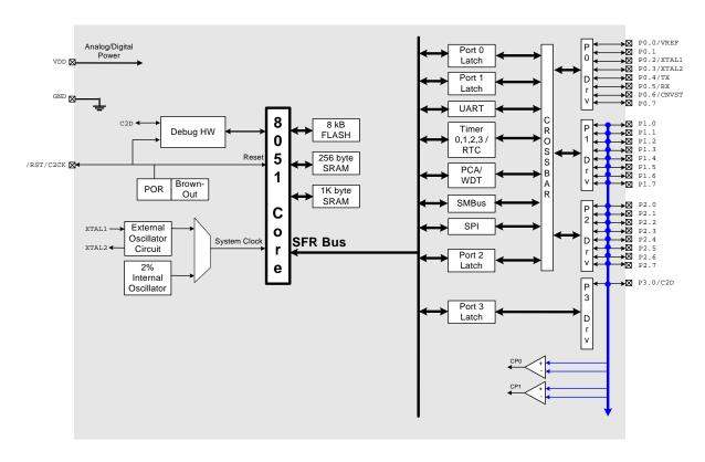
Figure 1.6. C8051F315 Block Diagram
