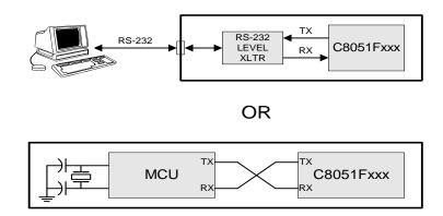
Figure 15.3. UART Interconnect Diagram
