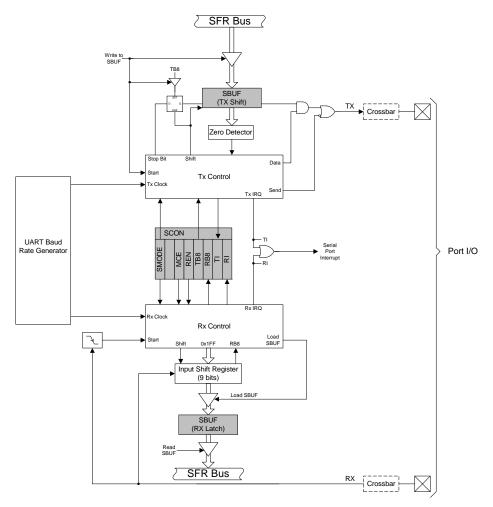
Figure 15.1. UARTO Block Diagram
