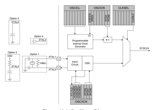
Figure 12.1. Oscillator Diagram
