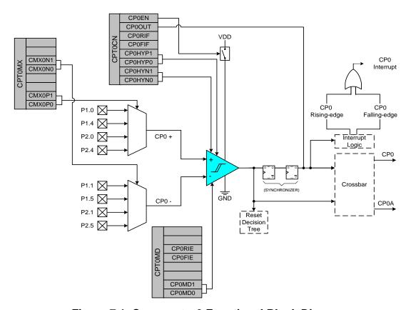
Figure 7.1. Comparator Functional Block Diagram
