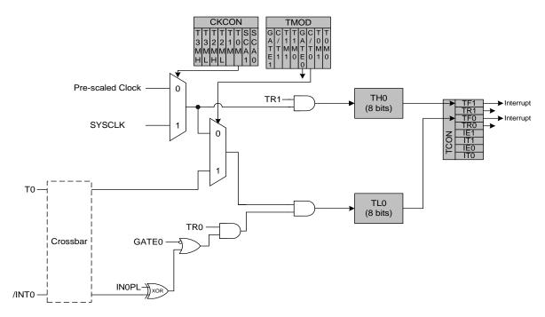
Figure 17.3. T0 Mode 3 Block Diagram
