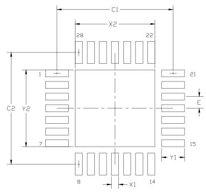
Figure 4.6. Typical QFN-28 Landing Diagram
