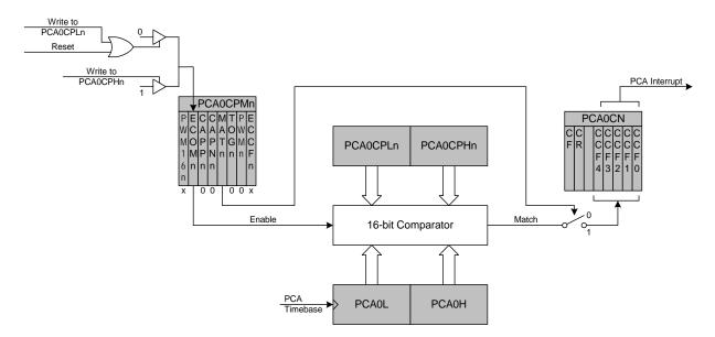
Figure 18.5. PCA Software Timer Mode Diagram
