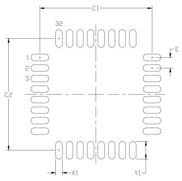
Figure 4.3. Typical LQFP-32 Landing Diagram
