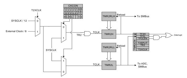
Figure 17.5. Timer 2 8-Bit Mode Block Diagram
