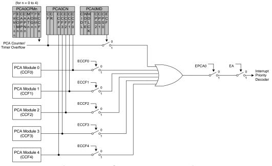
Figure 18.3. PCA Interrupt Block Diagram
