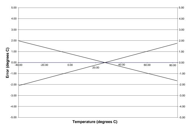
Figure 5.3. Temperature Sensor Error with 1-Point Calibration
