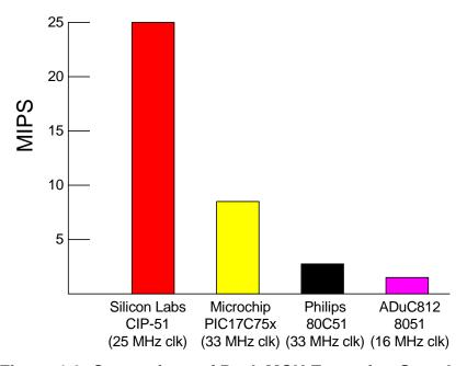
Figure 1.9. Comparison of Peak MCU Execution Speeds
