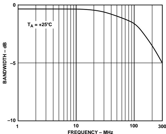
Figure 8. On Response vs. Frequency (B Grade)
