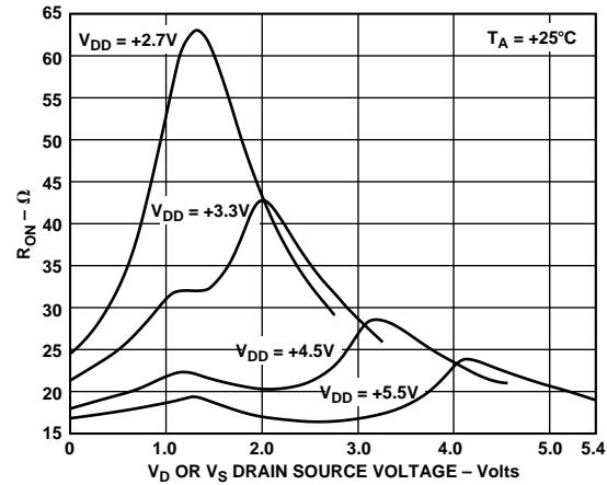
Figure 4. On Resistance as a Function of  $V_D$  ( $V_S$ ) Single Supplies (B Grade)
