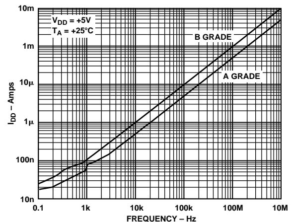
Figure 10. Supply Current vs. Input Switching Frequency
