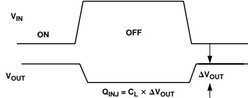
Test Circuit 5. Charge Injection
