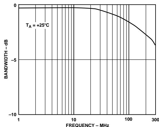
Figure 7. On Response vs. Frequency (A Grade)
