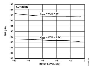
Figure 21. SNR vs. Input Level
