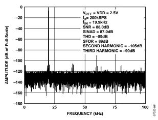
Figure 13. 20 kHz FFT,  $V_{REF} = VDD = 2.5 V$
