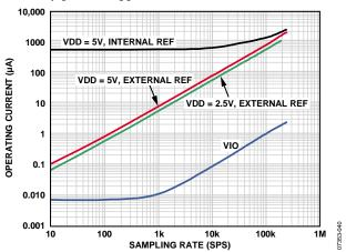
Figure 37. Operating Currents vs. Sampling Rate
