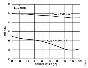
Figure 16. SNR vs. Temperature
