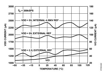
Figure 24. Operating Currents vs. Temperature
