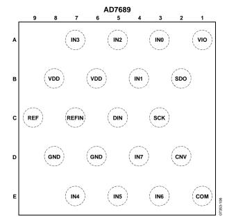
Figure 6. AD7682 WLCSP Pin Configuration
