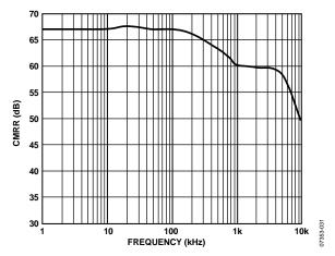
Figure 31. Analog Input CMRR vs. Frequency
