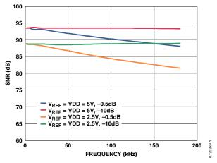
Figure 14. SNR vs. Frequency
