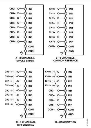
Figure 32. Multiplexed Analog Input Configurations
