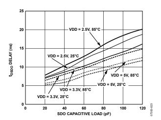
Figure 25. t<sub>DSDO</sub> Delay vs. SDO Capacitance Load and Supply
