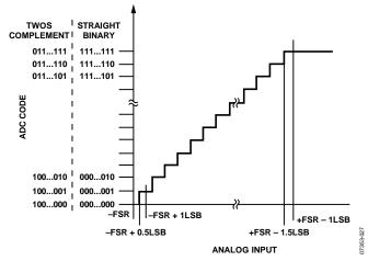
Figure 27. ADC Ideal Transfer Function
