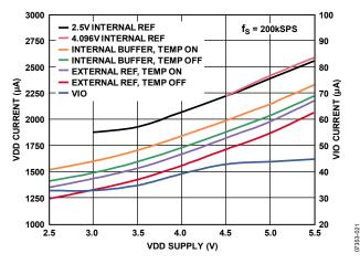
Figure 23. Operating Currents vs. Supply
