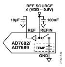
Figure 34. External Reference Using Internal Buffer
