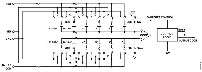
Figure 26. ADC Simplified Schematic
