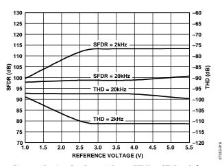
Figure 18. Spurious-Free Dynamic Range (SFDR) and THD vs. Reference Voltage
