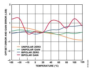
Figure 22. Offset and Gain Error vs. Temperature
