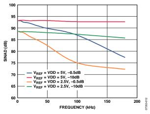
Figure 17. SINAD vs. Frequency
