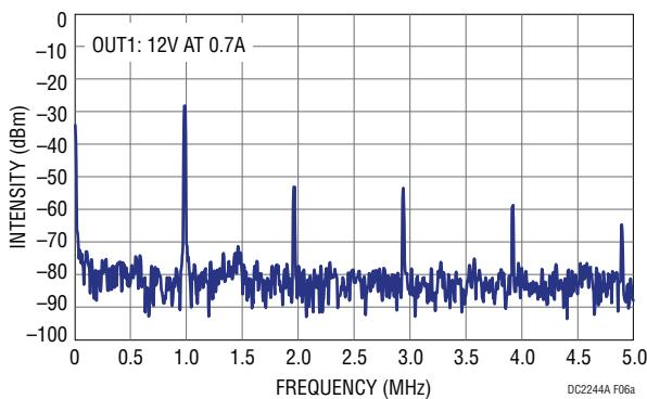
(a)  $V_{OUT1}$  Noise Spectrum,  $I_{OUT1} = 0.7A$
