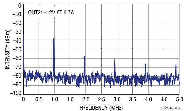
(b)  $V_{OUT2}$  Noise Spectrum,  $I_{OUT2} = 0.7A$ Figure 6. Output Noise Spectrum with 0.7A Load Current ( $V_{IN} = 12V$ , Short Output Ferrite Beads)
