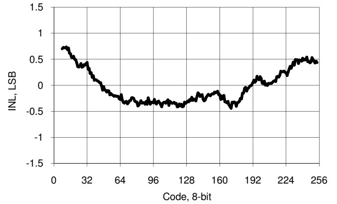
Figure 11-37. IDAC INL vs Input Code, Range = 255 \mu A, Sink Mode
