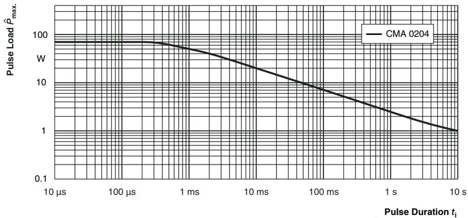
**Single Pulse** Maximum pulse load, single pulse; applicable if  $\bar{P} \rightarrow 0$  and  $n \leq 1000$  and  $\hat{U} \leq \hat{U}_{max}$ ; for permissible resistance change equivalent to 8000 h operation
