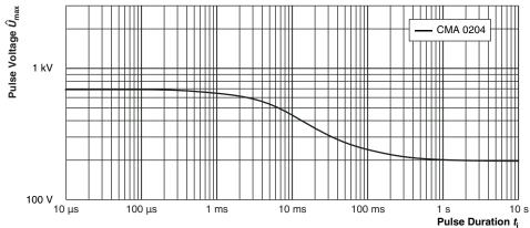
Maximum pulse voltage, single and continuous pulses; applicable if  $\hat{P} \le \hat{P}_{\max}$ ; for permissible resistance change equivalent to 8000 h operation
