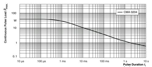
Maximum pulse load, continuous pulses; applicable if  $\bar{P} \leq P\left(\vartheta_{\rm amb}\right)$  and  $\hat{U} \leq \hat{U}_{\rm max}$ ; for permissible resistance change equivalent to 8000 h operation
