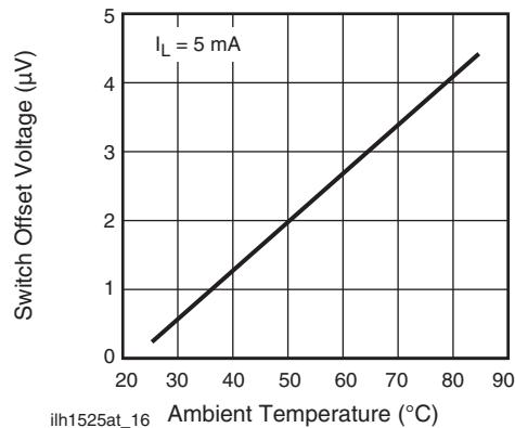
Fig. 17 - Switch Offset Voltage vs. Temperature
