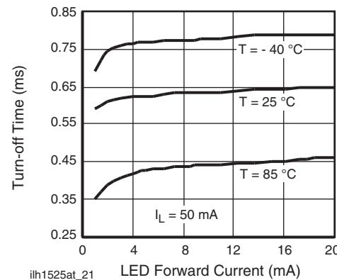
Fig. 22 - Turn-off Time vs. LED Current
