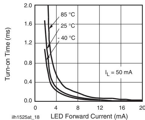
Fig. 19 - Turn-on Time vs. LED Current
