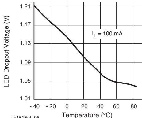
Fig. 7 - LED Dropout Voltage vs. Temperature
