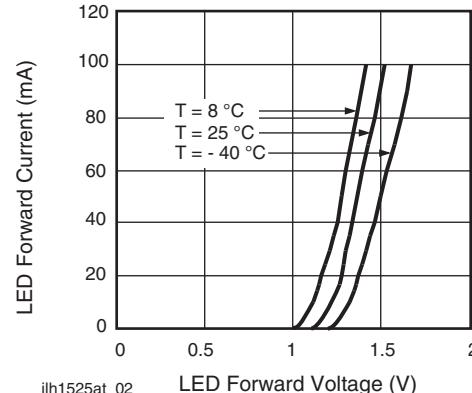
Fig. 3 - LED Forward Current vs. Forward Voltage
