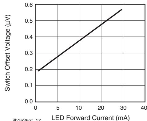
Fig. 18 - LED Offset Voltage vs. LED Current
