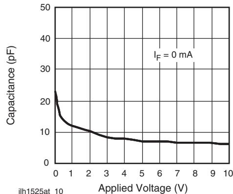
Fig. 11 - Switch Capacitance vs. Applied Voltage
