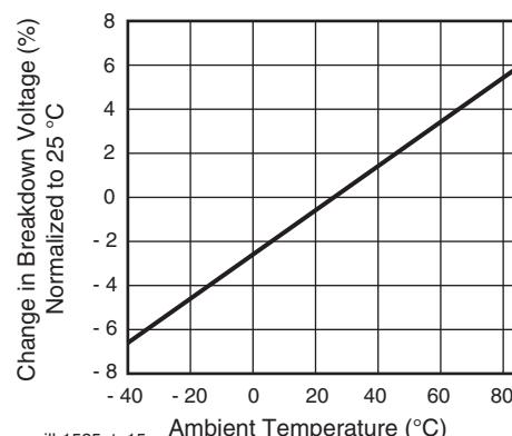
Fig. 16 - Switch Breakdown Voltage vs. Temperature
