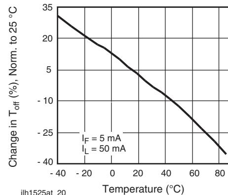
Fig. 21 - Turn-on Time vs. LED Temperature
