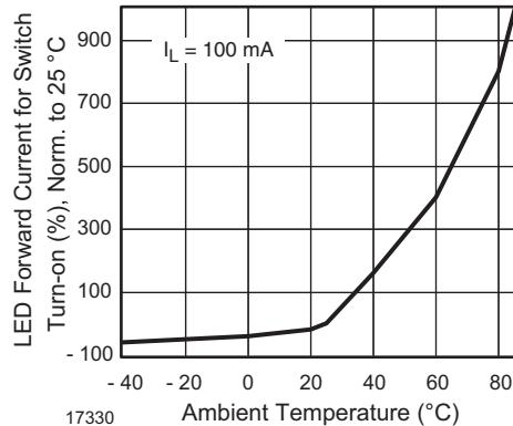
Fig. 5 - LED Current for Switch Turn-on vs. Temperature
