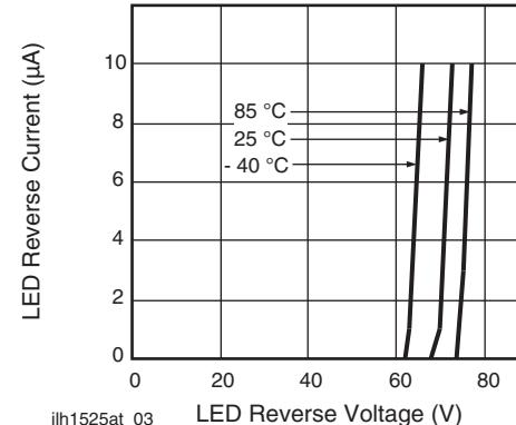
Fig. 4 - LED Reverse Current vs. LED Reverse Voltage
