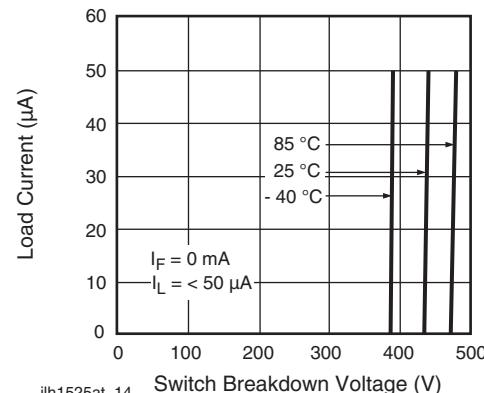
Fig. 15 - Switch Breakdown Voltage vs. Load Current
