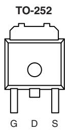
Drain Connected to Tab
