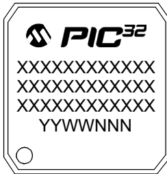
144-Lead TQFP (16x16x1 mm)
