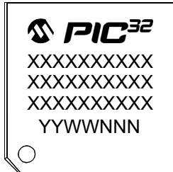
64-Lead TQFP (10x10x1 mm)
