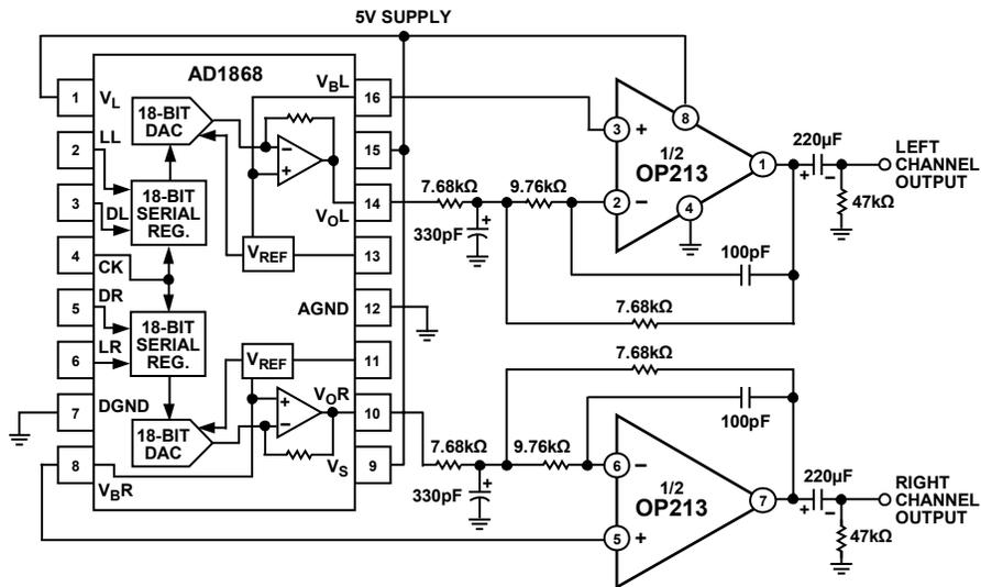
Figure 48. 5 V Only 18-Bit Stereo DAC
