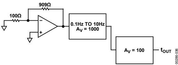
Figure 37. Noise Test Diagram
