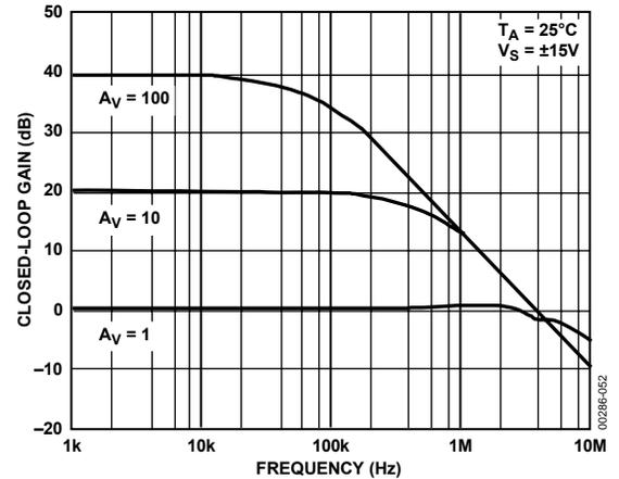
Figure 22. Closed-Loop Gain vs. Frequency @ ±15 V
