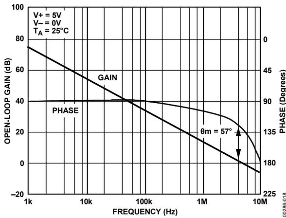
Figure 18. Open-Loop Gain, Phase vs. Frequency @ 5 V
