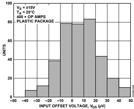
Figure 5. OP113 Input Offset ( $V_{OS}$ ) Distribution @  $\pm 15$  V
