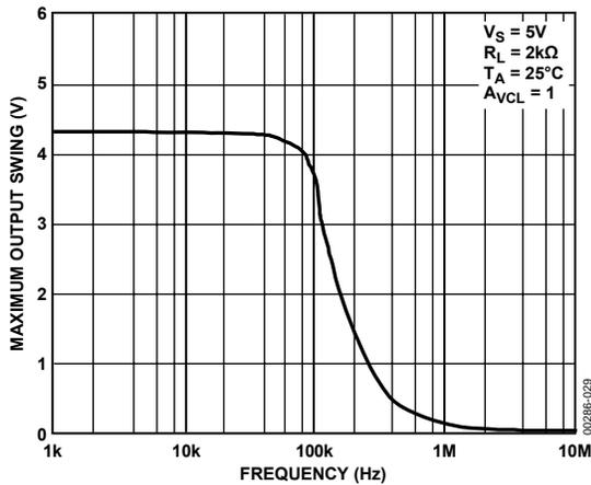
Figure 30. Maximum Output Swing vs. Frequency @ 5 V
