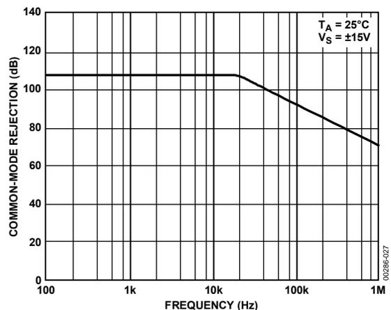
Figure 28. Common-Mode Rejection vs. Frequency @ ±15 V
