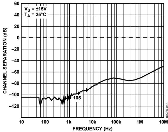
Figure 13. Channel Separation
