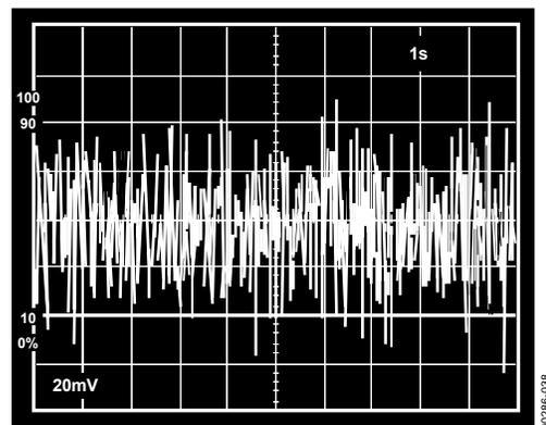
Figure 39. Input Voltage Noise @ 5 V (20 nV/div)
