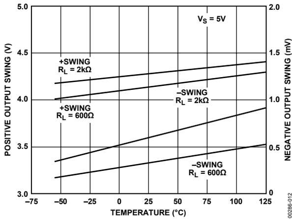
Figure 12. Output Swing vs. Temperature and  $R_L$  @ 5V
