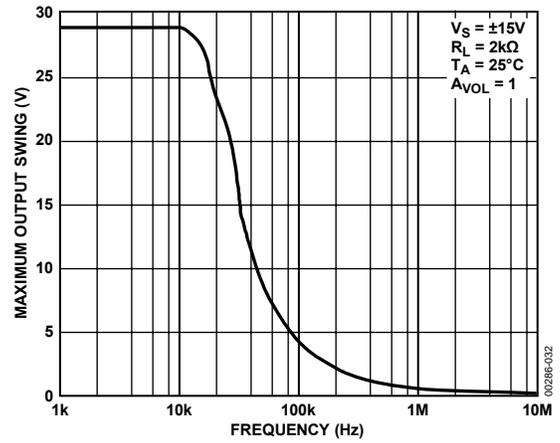
Figure 33. Maximum Output Swing vs. Frequency @ ±15 V
