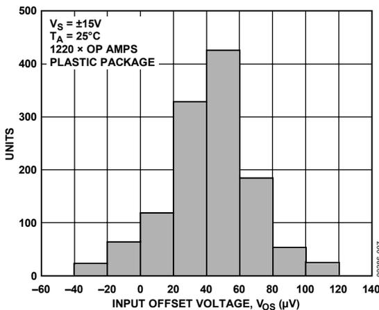
Figure 7. OP413 Input Offset ( $V_{OS}$ ) Distribution @  $\pm 15$  V
