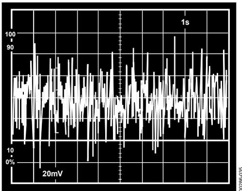
Figure 36. Input Voltage Noise @  $\pm 15\text{ V}$  (20 nV/div)
