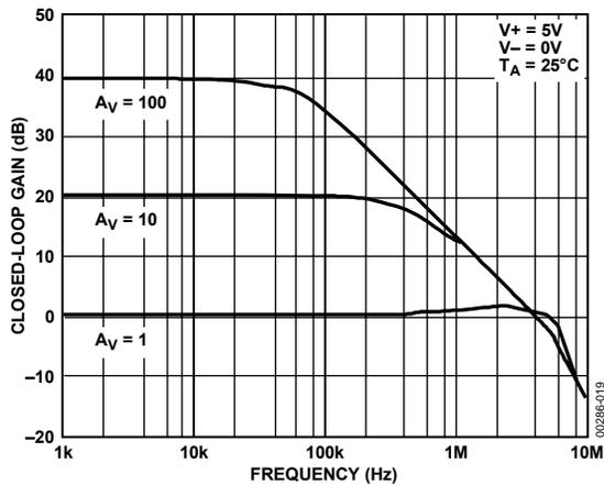
Figure 19. Closed-Loop Gain vs. Frequency @ 5 V
