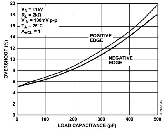
Figure 34. Small-Signal Overshoot vs. Load Capacitance @ ±15 V
