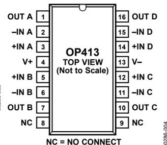
Figure 4. 16-Lead Wide-Body SOIC\_W
