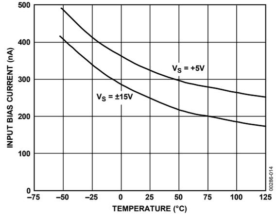
Figure 14. OP213 Input Bias Current vs. Temperature
