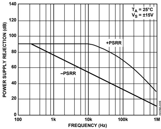
Figure 29. Power Supply Rejection vs. Frequency @ ±15 V
