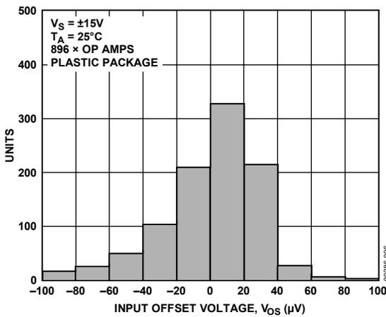
Figure 6. OP213 Input Offset ( $V_{OS}$ ) Distribution @  $\pm 15$  V
