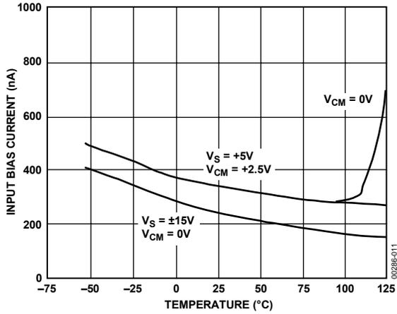
Figure 11. OP113 Input Bias Current vs. Temperature
