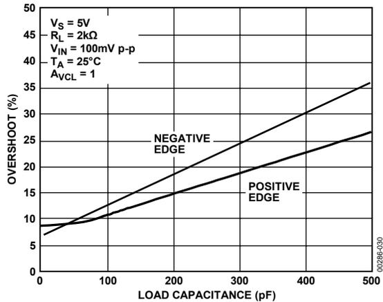
Figure 31. Small-Signal Overshoot vs. Load Capacitance @ 5 V
