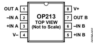
Figure 2. 8-Lead Narrow-Body SOIC\_N
