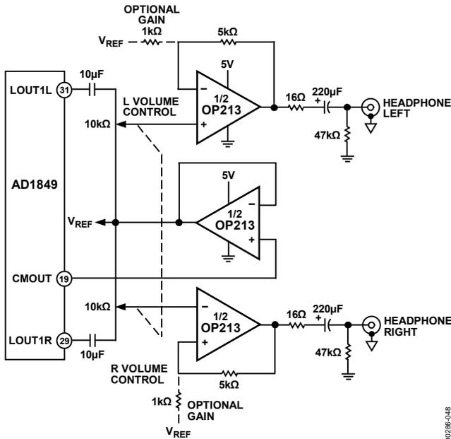
Figure 49. Headphone Output Amplifier for Multimedia Sound Codec
