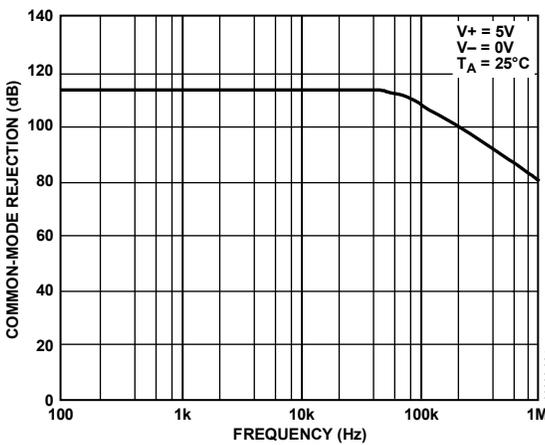
Figure 25. Common-Mode Rejection vs. Frequency @ 5 V
