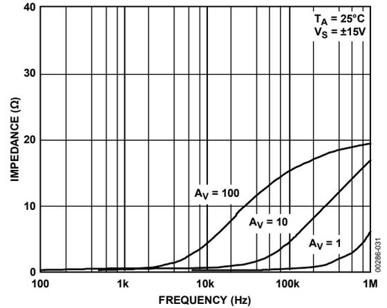
Figure 32. Closed-Loop Output Impedance vs. Frequency @ ±15 V
