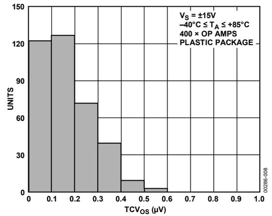
Figure 8. OP113 Temperature Drift ( $TCV_{OS}$ ) Distribution @  $\pm 15$  V
