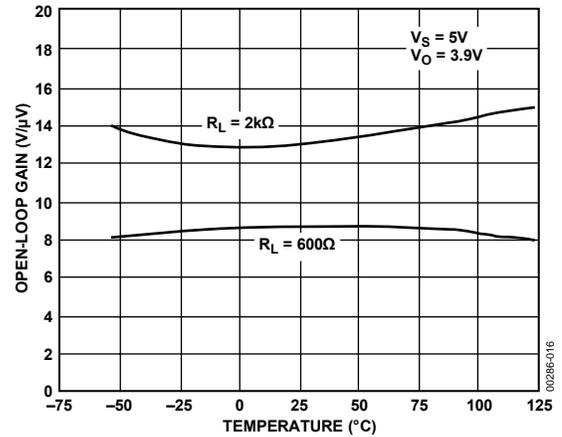
Figure 16. Open-Loop Gain vs. Temperature @ 5V
