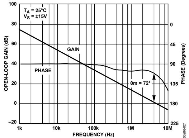
Figure 21. Open-Loop Gain, Phase vs. Frequency @ ±15 V
