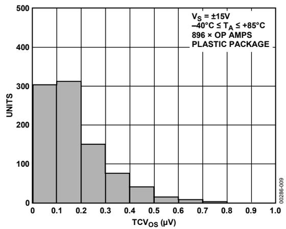
Figure 9. OP213 Temperature Drift ( $TCV_{OS}$ ) Distribution @  $\pm 15$  V
