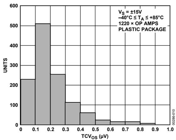
Figure 10. OP413 Temperature Drift ( $TCV_{OS}$ ) Distribution @  $\pm 15$  V
