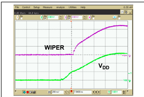
FIGURE 2-14: 2.1 k \Omega – Power-Up Wiper Response Time.
