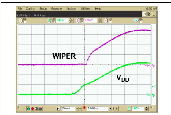
FIGURE 2-14: 2.1 k \Omega – Power-Up Wiper Response Time.
