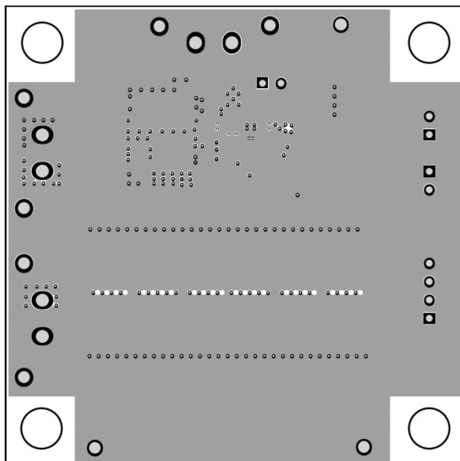
**Figure 8 – Layout GND**
