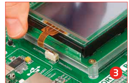
Figure 14-3: Now place GLCD with Touch panel into GLCD socket
