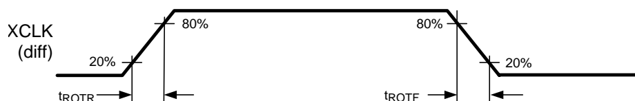
Figure 4. LVDS Output Transition Time
