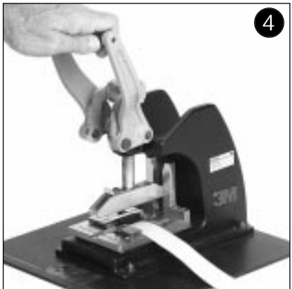
Lower the press handle to assemble the connector. It is recommended to check the tool setup before starting each production run. Proper seating of the connector cover onto the connector body can be checked by measuring the height of the connector/cover assembly.
