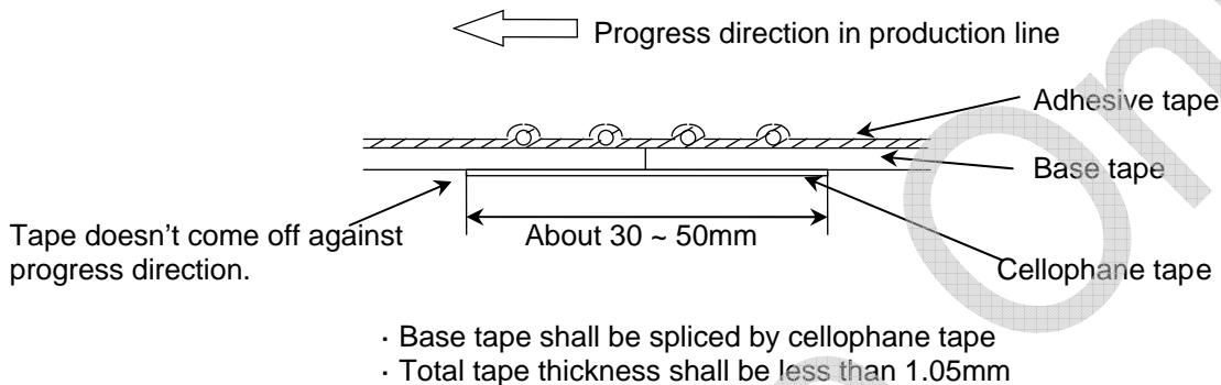
b. When adhesive tape is spliced :
