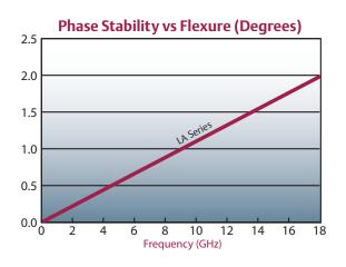
Phase stability is defined as the change in phase when the cable is bent 360 degrees around its minimum bend radius.
