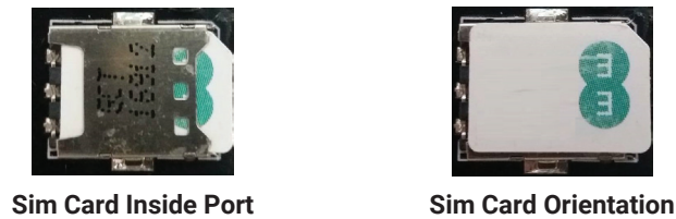
Figure 9 - Sim Card Orientation
