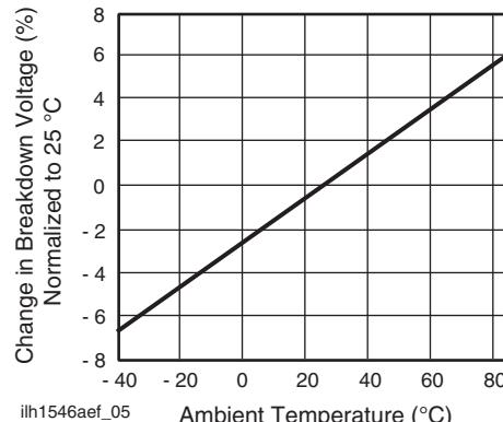
Fig. 4 - Switch Breakdown Voltage vs. Temperature
