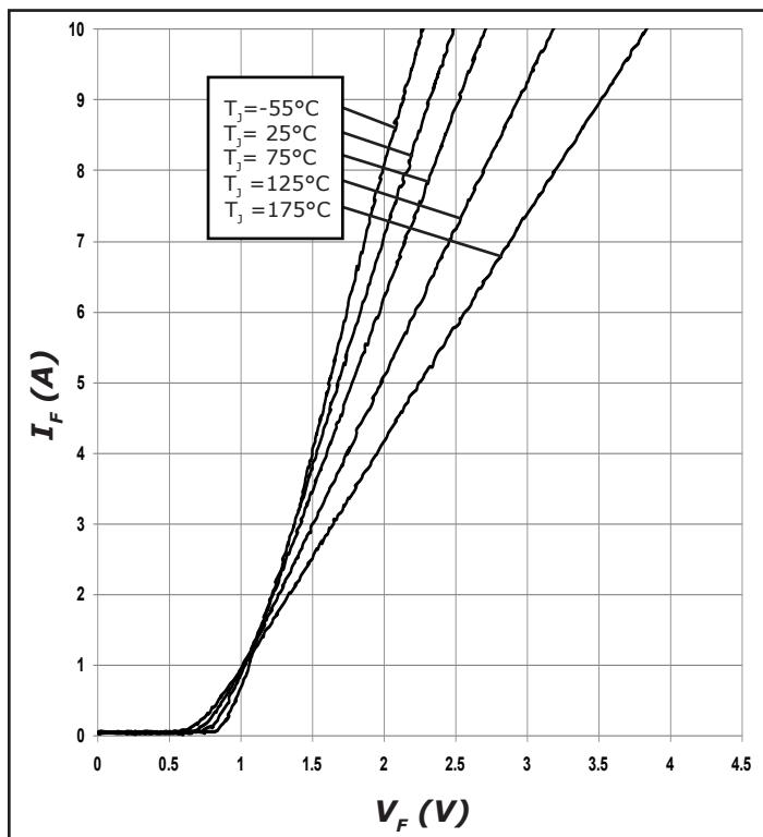
Figure 1. Forward Characteristics
