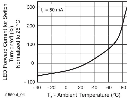
Fig. 5 - LED Current for Switch Turn-on vs. Temperature
