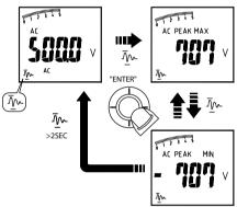
2. In AC A mode, select "小☆" indicator then press the navigator key for more than 2 seconds to enter PEAK HOLD mode. To exit PEAK HOLD mode, just press the navigator key for more than 2 seconds to return to the "小☆" indicator.
