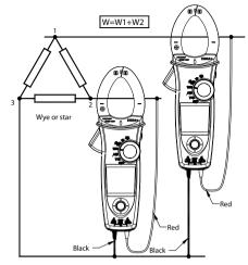
**B.** 3 phase 4 wire balanced / unbalanced *Step1*. Set the rotary switch to the "W" position *Step2*. Using the Navigator key to choose the "W" mode.
