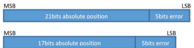
Figure 10: AR35 SSI 3-Wire Format Output
