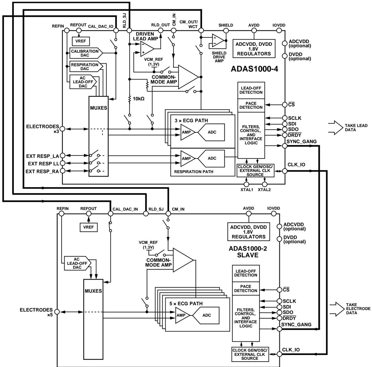
Figure 74. Configuring Multiple Devices to Extend Number of Electrodes/Leads
