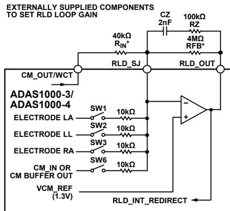
\*EXTERNAL RESISTOR R<sub>IN</sub> IS OPTIONAL. IF DRIVING RLD FROM THE ELECTRODE PATHS, THEN THE SERIES RESISTANCE WILL CONTRIBUTE TO THE R<sub>IN</sub> IMPEDANCE. WHERE SW1 TO SW5 ARE CLOSED, R<sub>IN</sub> = 2kΩ. RFB SHOULD BE CHOSEN ACCORDINGLY FOR DESIRED RLD LOOP GAIN.
