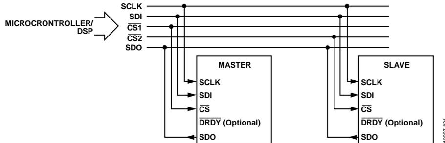
Figure 75. One Method of Interfacing to Multiple Devices
