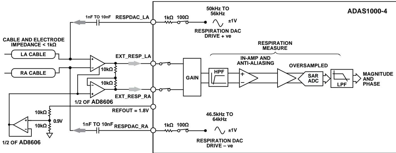
Figure 69. Respiration Using External Capacitor and External Amplifiers
