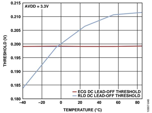
Figure 20. DC Lead-Off Comparator Low Threshold vs. Temperature
