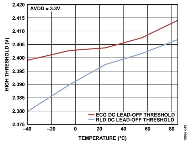
Figure 21. DC Lead-Off Comparator High Threshold vs. Temperature
