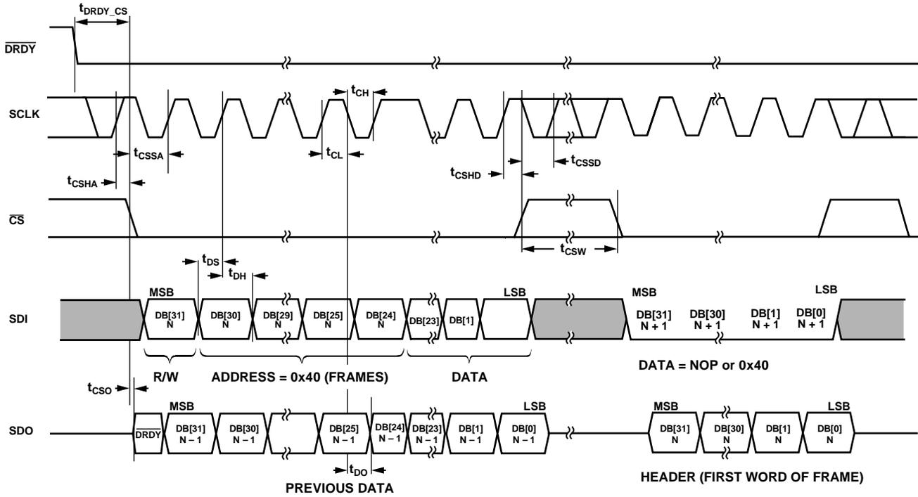
Figure 3. Starting Read Frame Data (CPHA = 1, CPOL = 1)
