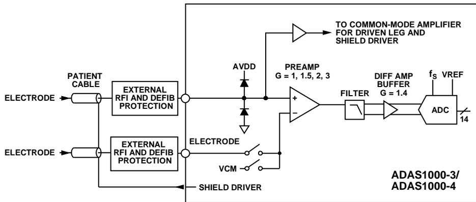
Figure 54. Simplified Schematic of a Single ECG Channel
