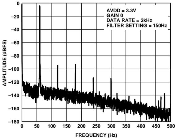
Figure 47. FFT with 60 Hz Input Signal
