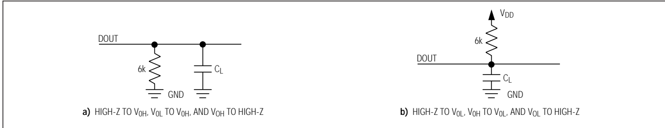
Figure 1. Load Circuits for Enable and Disable Time
