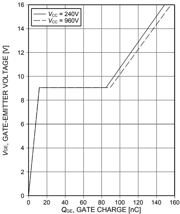
Figure 14. **Typical gate charge**
