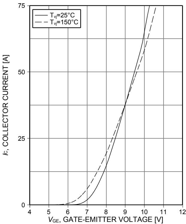
Figure 5. Typical transfer characteristic
