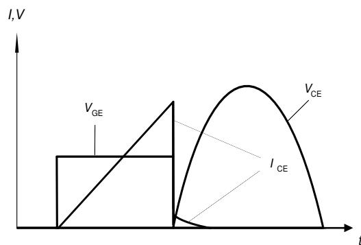
Figure C. Typical switching behavior in resonant applications
