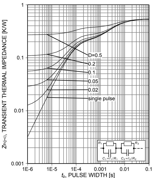
Figure 16. **IGBT / Diode transient thermal impedance**
