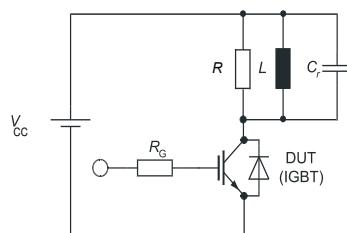
Figure E. Dynamic test circuit
