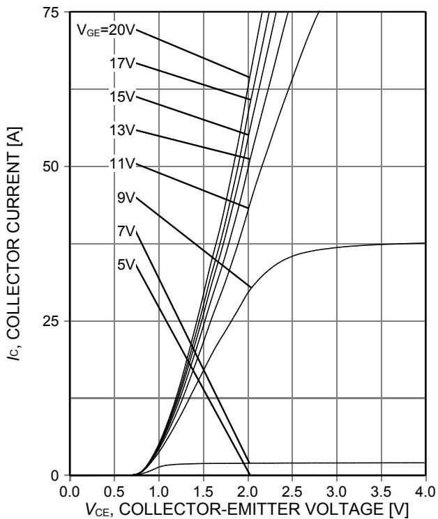
Figure 3. Typical output characteristic
