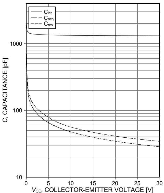
Figure 15. **Typical capacitance as a function of collector-emitter voltage**
