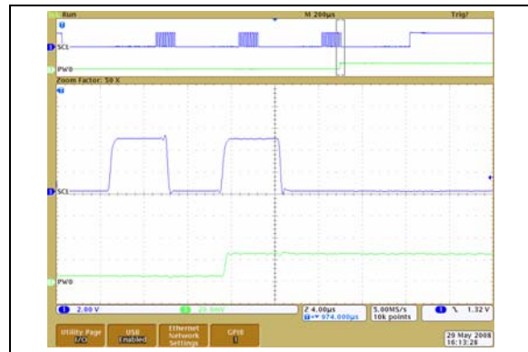
FIGURE 2-44: 50 k \Omega – Low-Voltage Increment Wiper Settling Time ( V_{DD} = 2.7\text{V} ) (1 \mu\text{s}/\text{Div} ).
