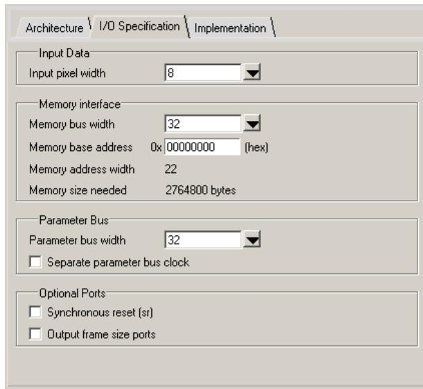
**Input pixel width** sets the bit width of the incoming pixel. Values can be 8, 10 and 12. Default value is 8.
