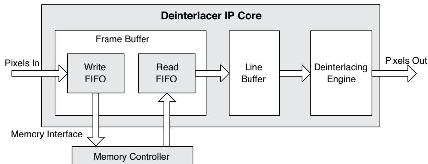
Figure 2-1 shows the block diagram of the Deinterlacer IP core. The core consists of three modules: frame buffer, line buffer and deinterlacer engine. The frame buffer module manages memory write/read and combines interlaced fields into progressive frames. The line buffer module and deinterlacing engine process the combined frames to reduce artifacts.
