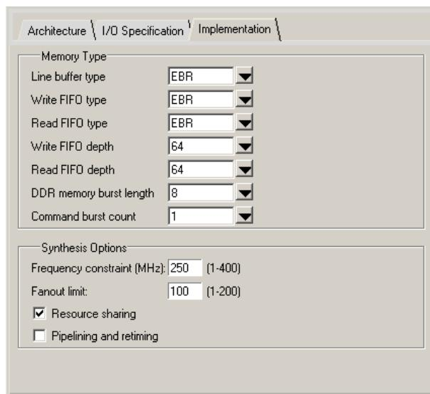
**Line buffer type** selects EBR or Distributed RAM for the line buffer implementation.
