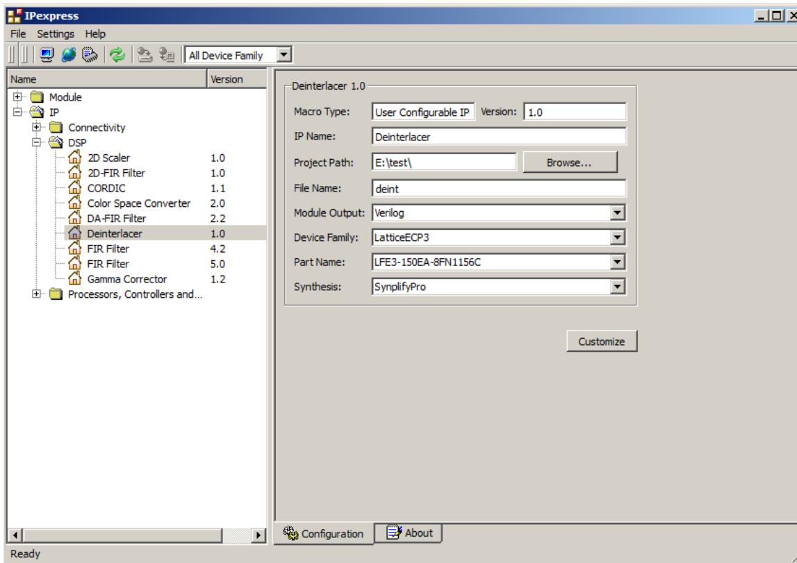
**Important Note:** File Name cannot be “deinterlacer\_core,” as this name has been used in the internal design of the core.
