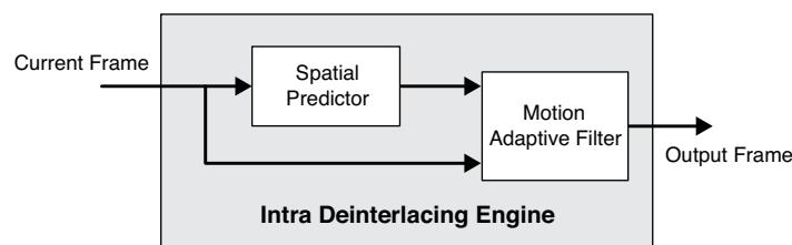
Figure 2-2 shows the structure of the intra deinterlacing engine.
