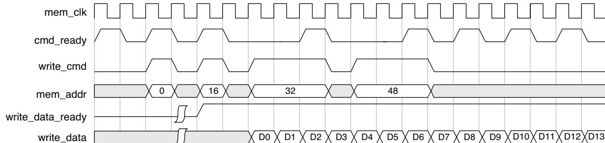
Figure 2-13 shows the timing of the memory read operation. When the internal read FIFO is less than half full, and there is no ongoing write operation, memory read burst operation is started. The length of the read burst operation and once read burst makes the read FIFO half full.
