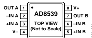
Figure 4. 8-Lead MSOP (RM-8)
