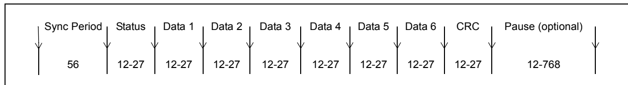
FIGURE 16-2: SENTx PROTOCOL DATA FRAMES
