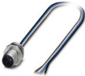
Sensor/Actuator flush-type plug, 4-pos., M12, A-coded, front/screw mounting with PG9 thread, with 0.5 m TPE litz wire, 4 x 0.34 mm²
