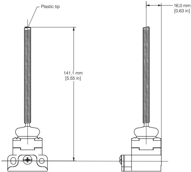
Figure 14. Plastic Rod and Flexible Cable
