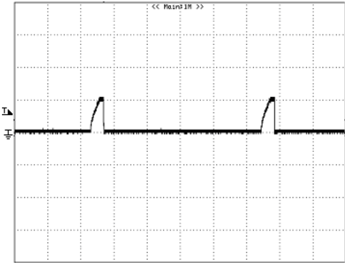
Figure 21: Output short circuit current 5V_{in} , 0.75V_{out} 20A/div , 10mS/div
