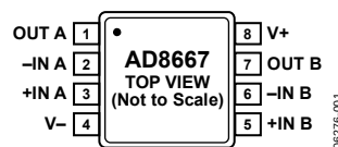
Figure 1. 8-Lead MSOP, 8-Lead SOIC
